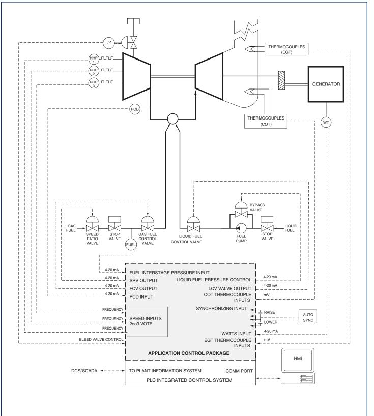
Simplified schematic showing a Petrotech Fiat TG16<sup>®</sup> gas turbine generator drive application control package integrated into an advanced PLC-based control system. Shown with dual fuel system.
