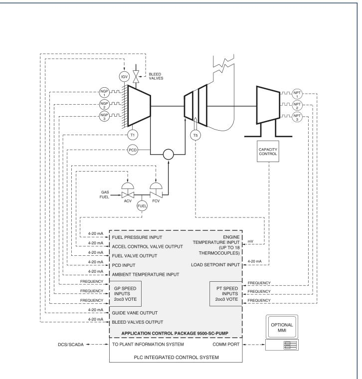
Simplified schematic showing a Petrotech Solar Centaur® pump drive application control package integrated into an advanced PLC-based control system.
