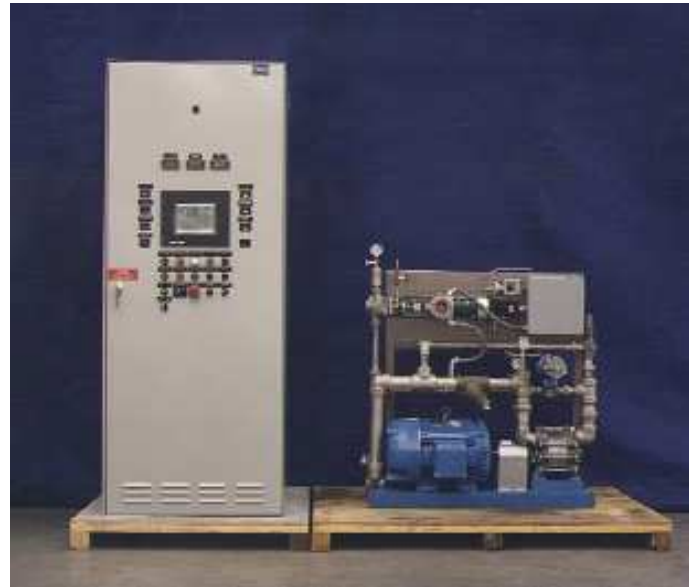
Replacement controls for one GE Frame 5 gen set in utility peaking service with water injection skid for NOx reduction.
