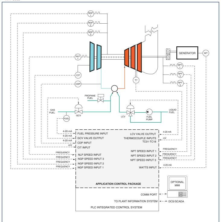
Simplified schematic showing a Pratt & WhitneyGG4 gas turbine generator drive application control package integrated into an advanced PLC-based control system.
