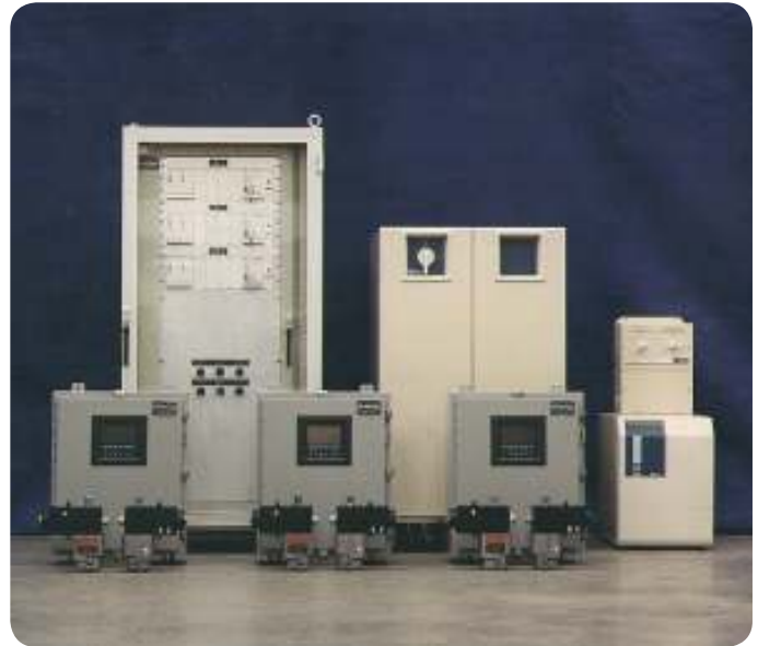
Compressor capacity control system upgrade for three units, featuring HydroCOM actuators with stepless torque control system, local control panels, RS485 network, and UPS backup power system.
