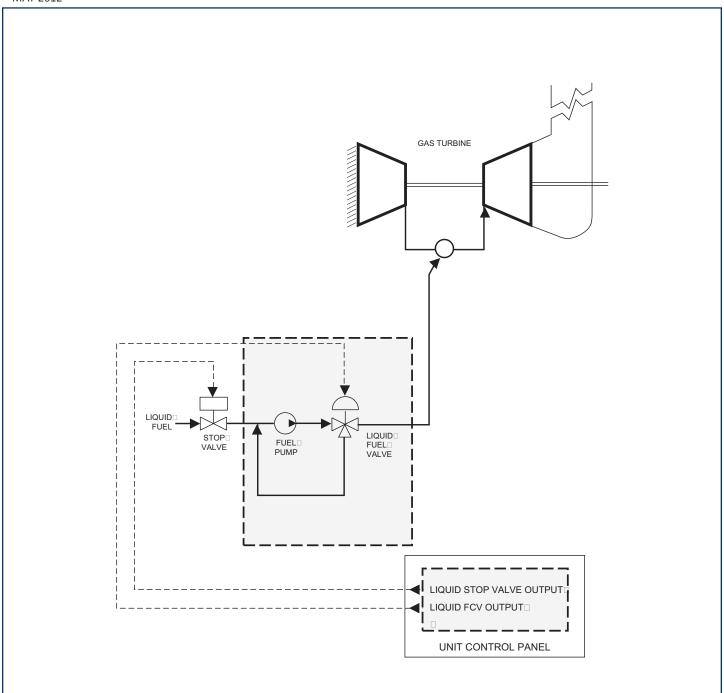
Simplified schematic showing principal parts of the Petrotech gas turbine liquid fuel system upgrade, universal fuel system design.
