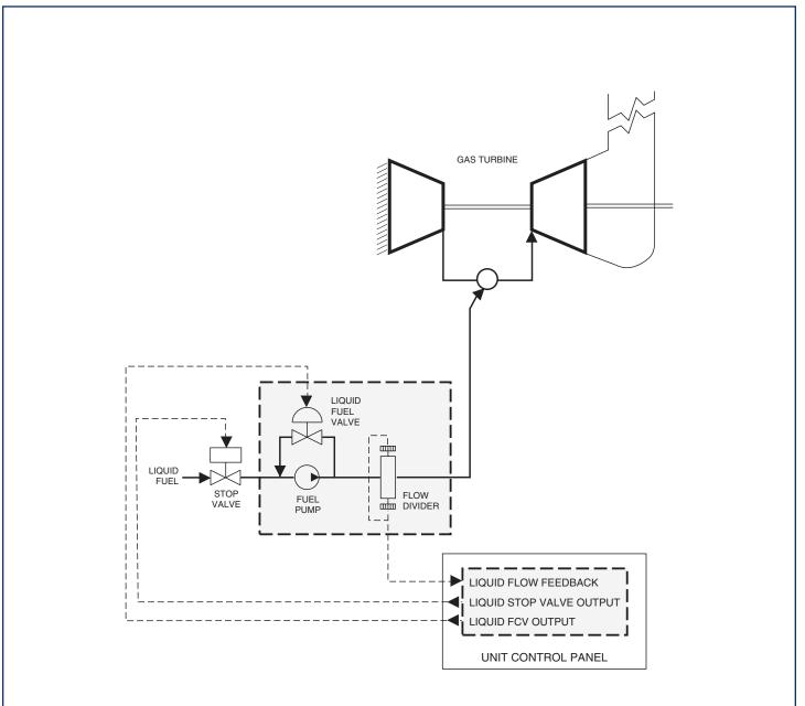
Simplified schematic showing principal parts of the Petrotech gas turbine liquid fuel system upgrade, universal fuel system design.
