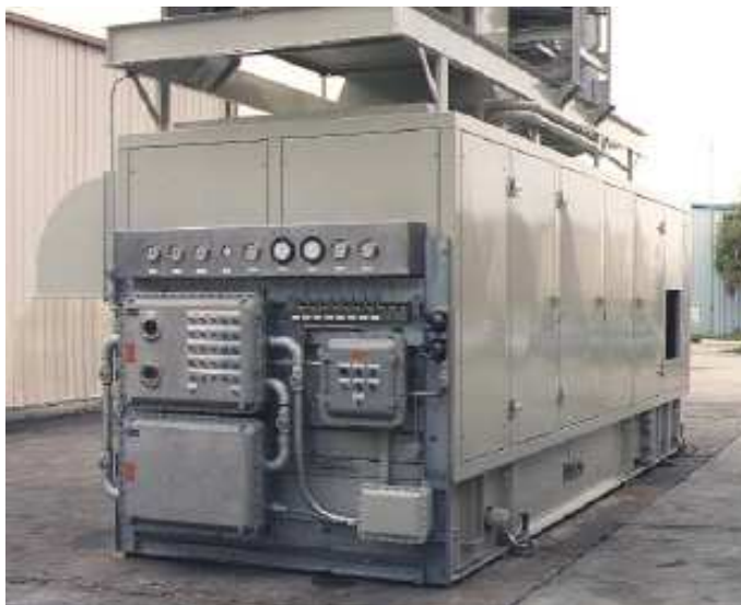
Explosion proof Division 2 replacement controls for Solar Centaur in offshore gas gathering service
